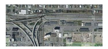
FIGURE 36: Single Point Urban Interchange (SPUI)
