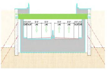
**FIGURE 18:** Depressed Highway with Cantilevered City Streets, Queens, NY
