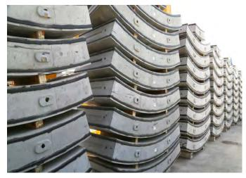
FIGURE 25: Precast Segments for Eurasia Tunnel, Turkey
